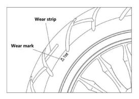
Fig12 Inspection of the tire
