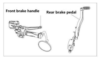
Fig16 Brake position diagram
