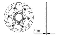
Fig26 Front brake disc inspection
