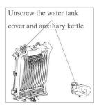
Fig 36 Adding coolant
