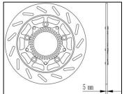
The brake disc will gradually wear out during long-term use, so it is necessary to check the thickness dimension of the brake disc at multiple positions. And inspect its appearance to confirm whether the brake disc is damaged, cracked, or deformed.
