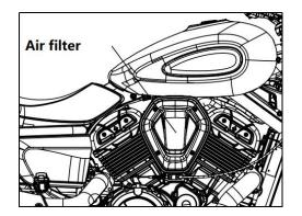
Fig20 Air filter position
