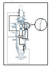
ABS consists of hydraulic unit, ABS control unit, and return pump, installed under the seat. There are two wheel speed sensors on the front and rear wheels.
