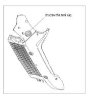
Fig35 Adding coolant
